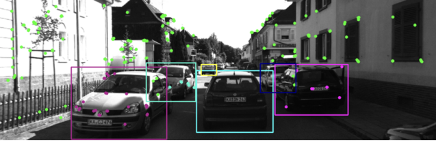
Fig. 5: Object association in the dynamic and occluded scenarios of KITTI 07. Green points are the non-object points, and points in other colors are associated with objects of the same color. The front cyan moving car is not added as a SLAM landmark as no feature point is associated with it. Points in object overlapping areas are not associated with any object due to ambiguity.
